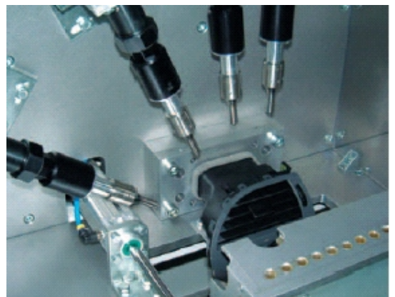
Special purpose machine for welding of air nozzle mounting hooks around periphery.
